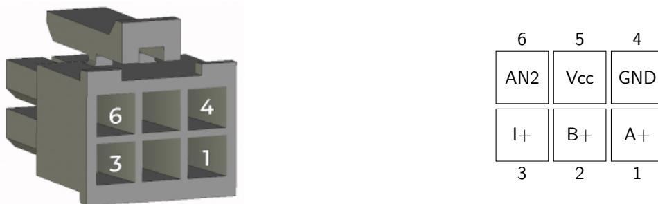
Figure 1.11: J401 pins, 2 x 3 pins, auxiliary sensor input
