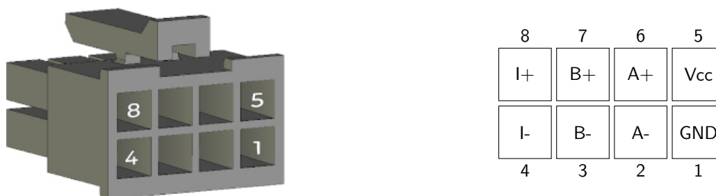
Figure 1.8: J301 pins, 2 x 4 pins, main sensor input
